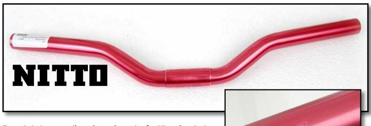
**Euro-Asia Imports,** the primary importer for **Nitto Co., Ltd.** in North America, is voluntarily recalling Nitto aluminum bicycle handlebars with model number **B259AA**. The bicycle handlebars can break, resulting in loss of control and a fall hazard.
